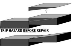
TRIP HAZARD AFTER SAW CUT REPAIR
