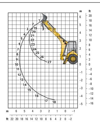
Lift capacities are over-end values calculated according to SAE J31. Values are 87% of the maximum lift force available. Machine equipped with AWD, OROPS, 0.96 m<sup>3</sup> (1.25 yd<sup>3</sup>) general purpose bucket and no counterweight. Extendible stick includes 460 kg (1,015 lb) counterweight.
